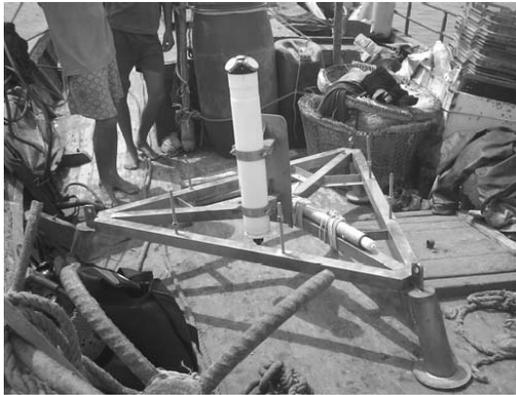
Figure 4: Argonaute ADP (Acoustic Doppler Velocimeters)
