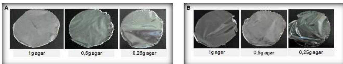
Figure 2: Commercial (A) and algal (B) bioplastic with different agar contents
