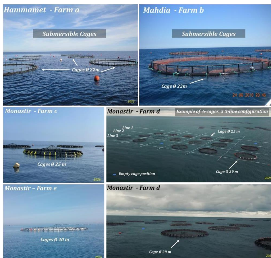
Figure 5. Examples of Submersible and Surface floating Cage systems and Multi-Line Cage Configurations observed in Tunisian Aquaculture Far.
